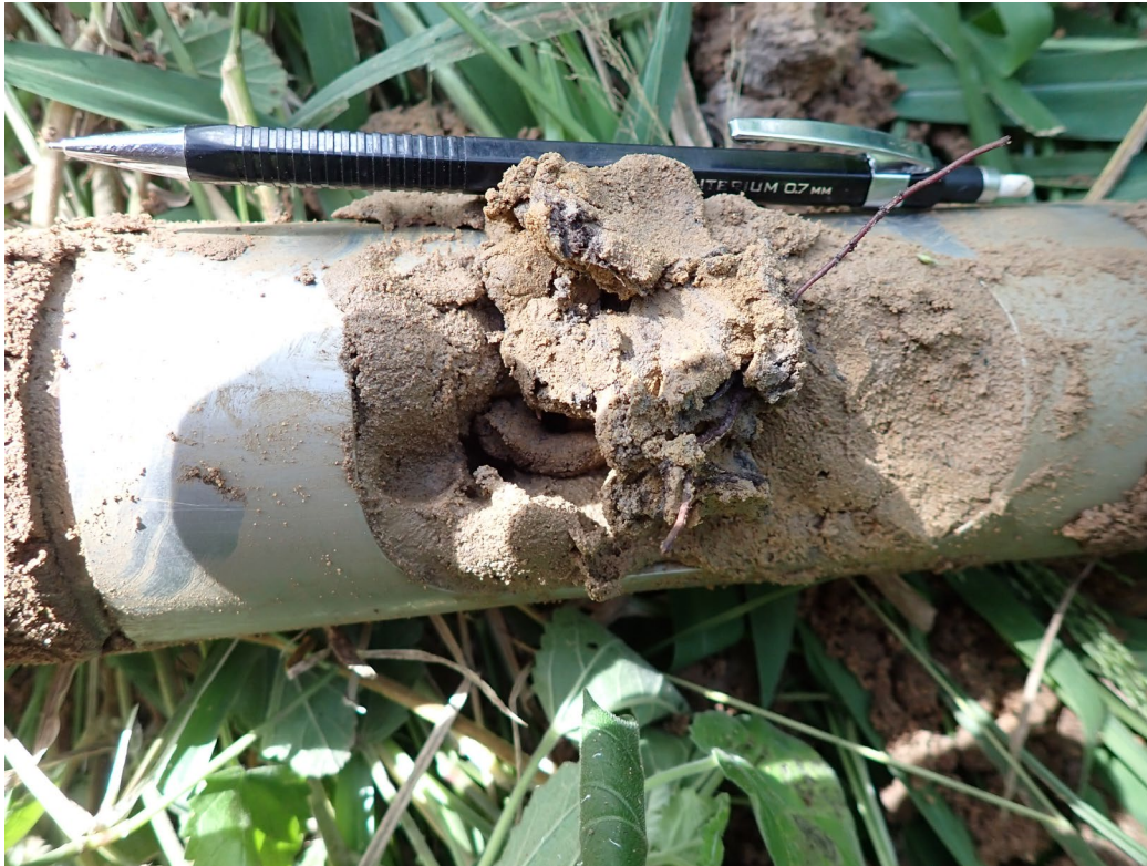
Photograph 4. Coarse tree roots intersected at 3.8mbgl at Site 13 auger 2 (S13_AU2), located immediately above the water table.
