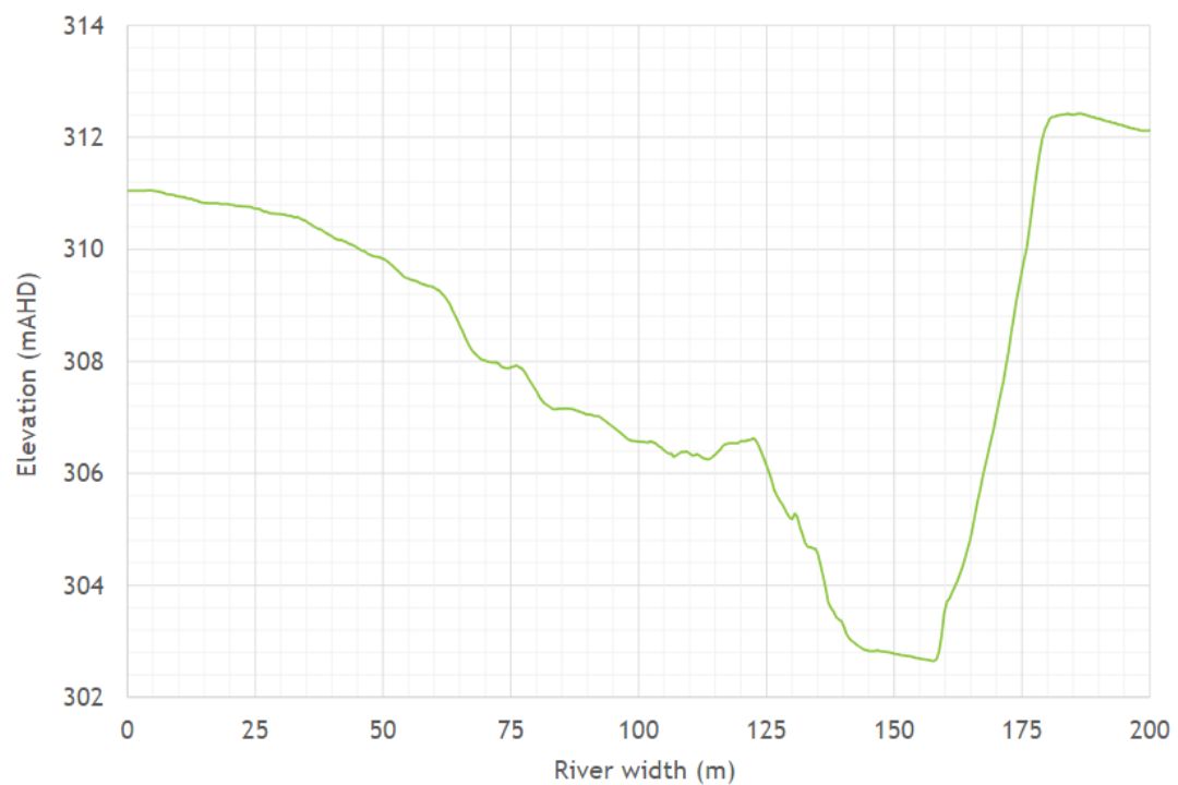
Figure 3.15 Isaac River typical cross-section in the Project area – showing benching along straight river sections
