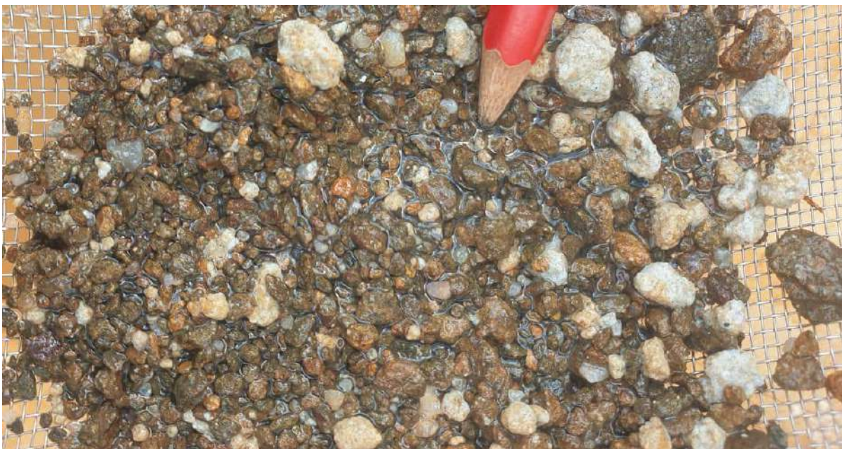
Figure 2 Very weathered sandstone, Anna Creek Downstream 15-15.4m
