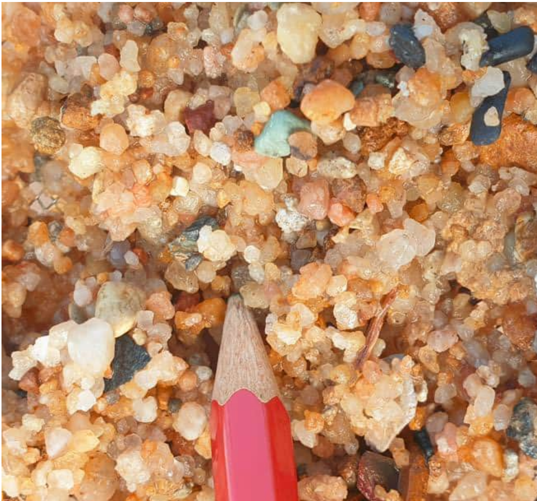
Figure 1 Coarse rounded sand max 0.5cm, Anna Creek Downstream 10-12m.
