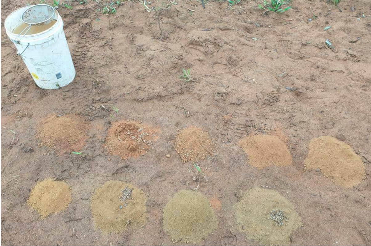
Figure 4 Drill cuttings of Teviot Creek up-stream, progress from top left to bottom right. Weathered sandstone from about 7m onwards.
