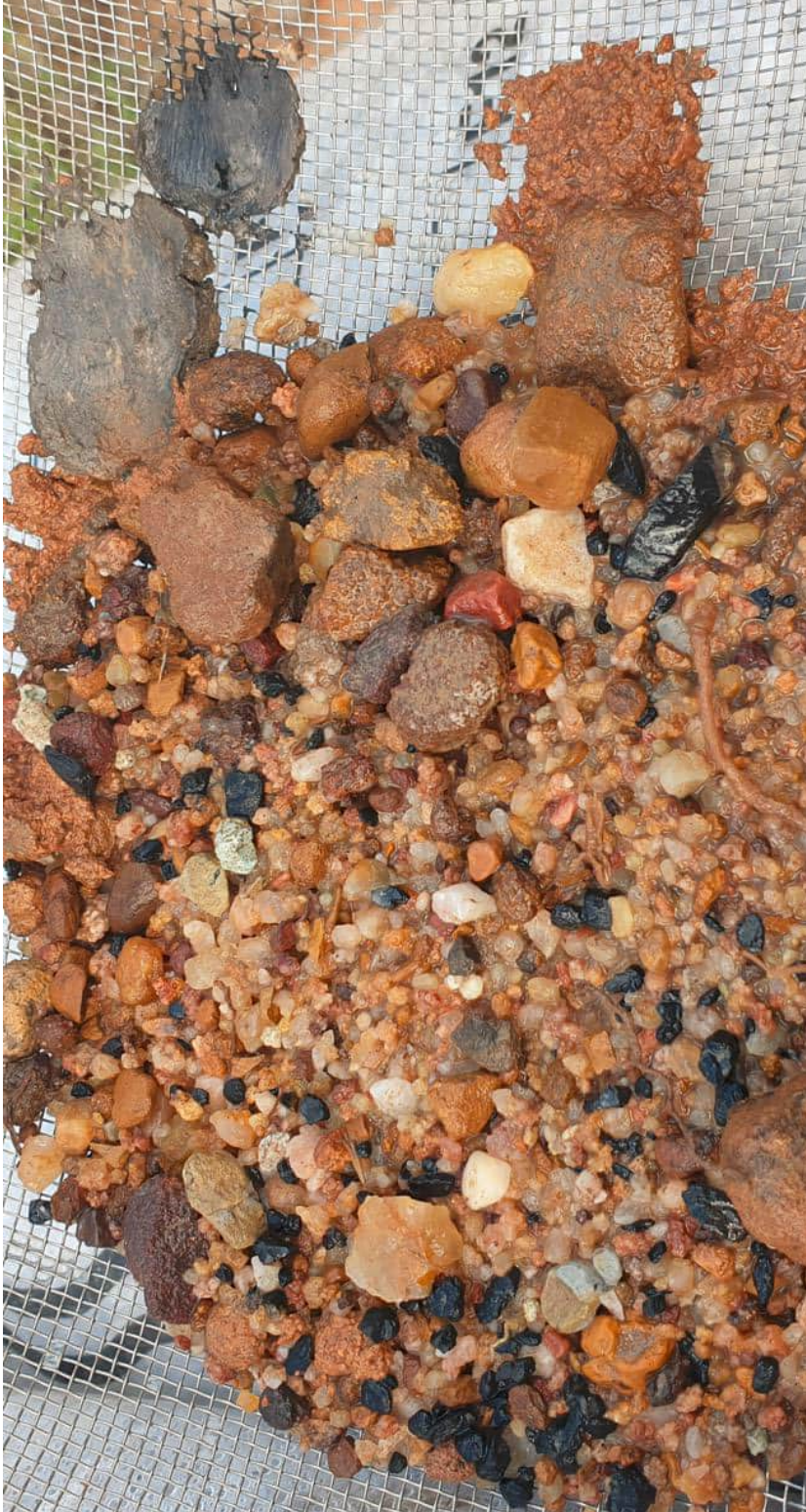
Figure 3 Teviot Creek Downstream. 16-17m, dark grey plastic clay + coal in alluvial wash from strata above
